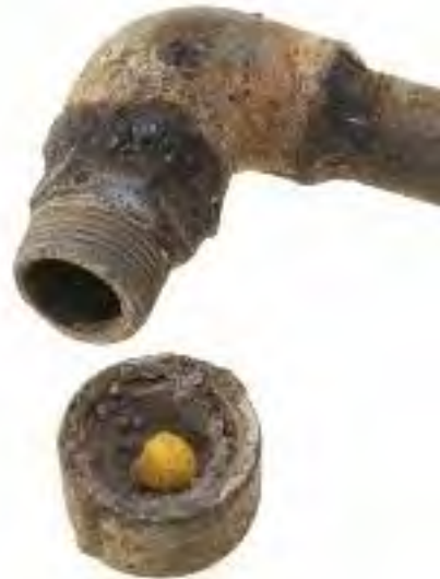
Figure 29 D. Most of the mercury has evaporated and the gold is left behind.
