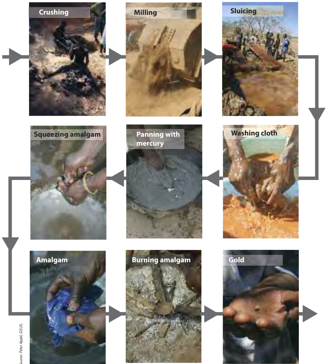
Figure 27. Flowchart. Gold extraction using mercury. Amalgamation Process.
