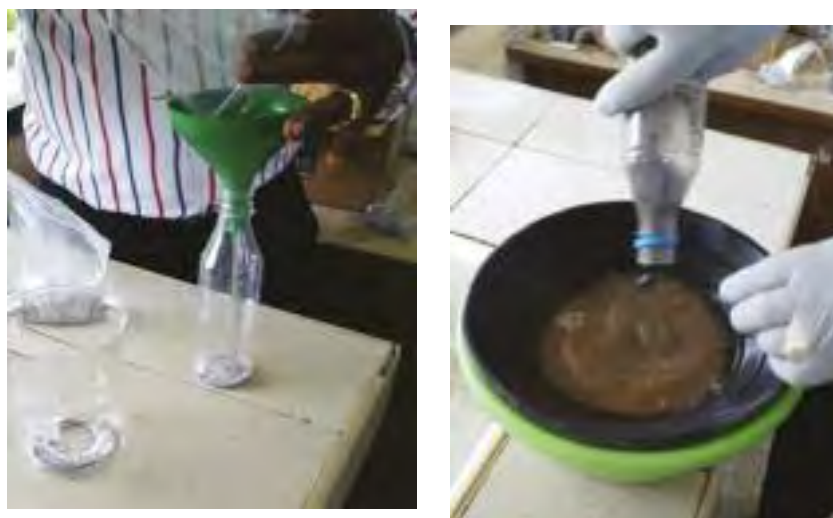
Figure 28. Safer alternative to separate Amalgam from black sands.
