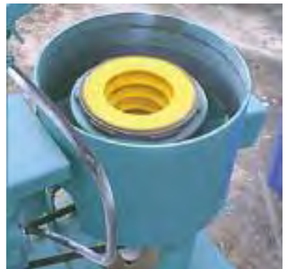
Fig. 26. Example of a Separating Bowl of a Centrifugal Concentrator.
