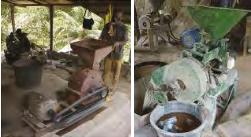
Fig. 20. Hammer mill and disc mill at Takote Mine in Western Ghana.
