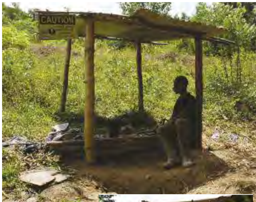
Figure 30. The retorting is carried out at some distance from the mining site due to the danger of mercury vapor.
