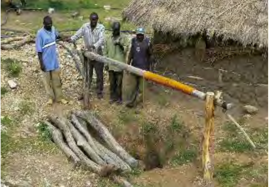
Figure 11. ASM Operators Using a Winch to Raise Material From a Deep-Shaft Mine.
