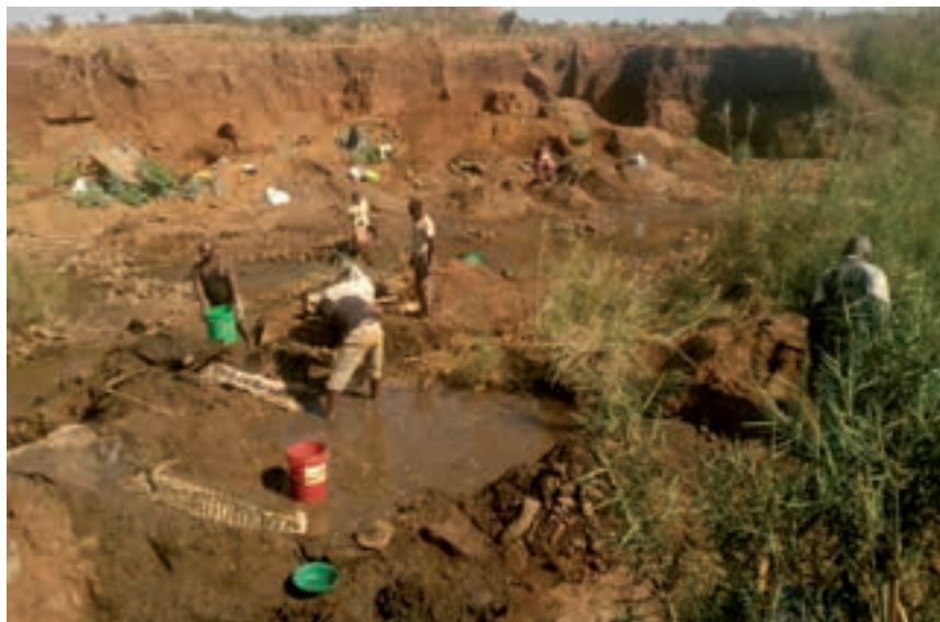
Figure 15. Alluvial Gold Sluicing Using Sluicing Board Along the Natherenje River, Central Malawi
