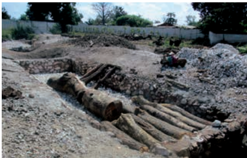
Figure 9: A Traditional Batch Kiln for Limestone Combustion
