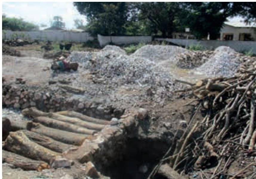
Figure 20. Limestone Burning in a Rectangular-Type Kiln
