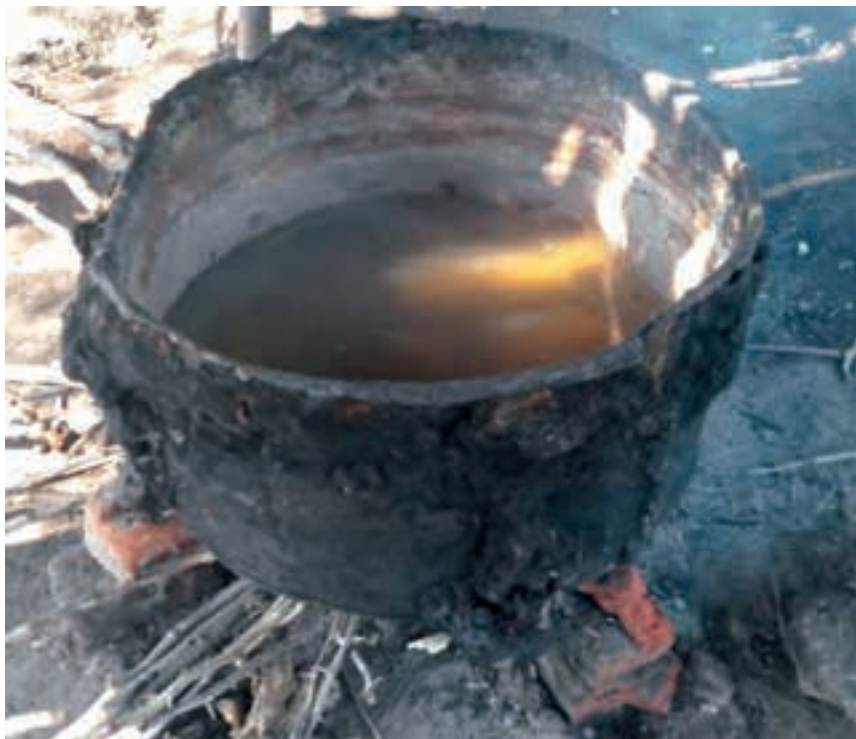
Figure 12. Brine Boiling Process to Enable Salt Crystallisation
