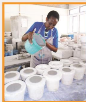
Forming by slip casting
