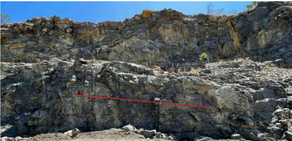
Figure 17 - Scanline in the rock slope outcropping in the Njuli Quarry
