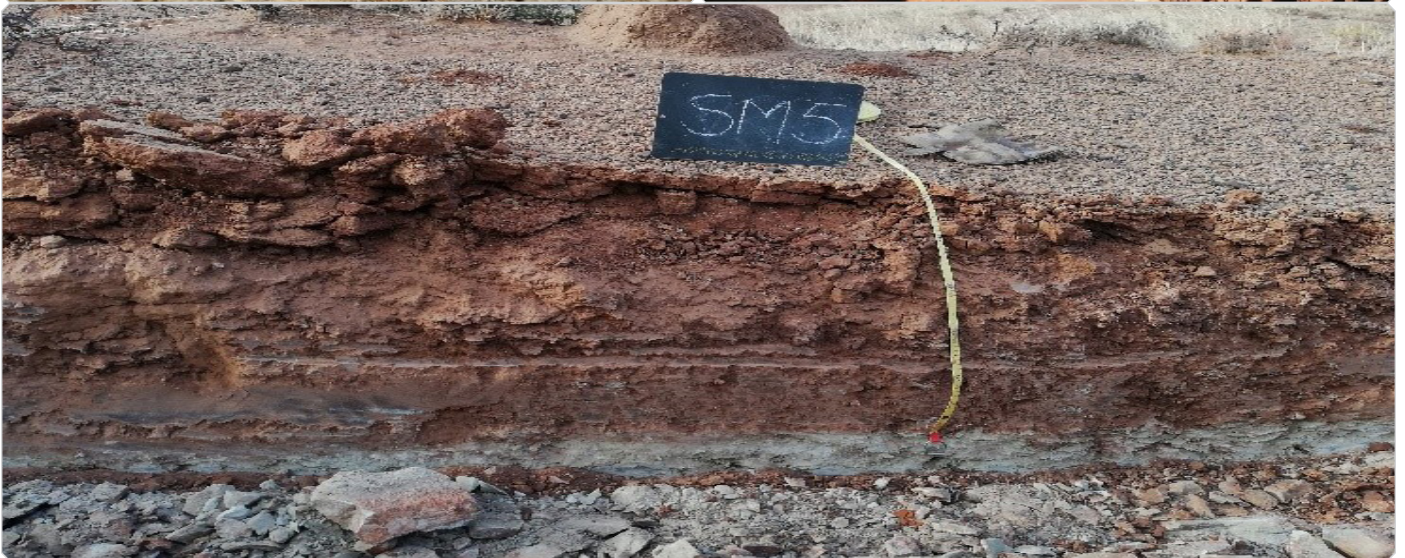
Photographs of various geotechnical site investigation activities and exposed profiles during fieldwork. Top: TLB excavation of an exploratory hole in progress. Top and middle left and right photos: transported fine colluvium (hillwash) overlying interbedded sandstone-mudrock bedrock. Bottom photo: imported fill, overlying fine alluvium and residually weathered sandstone.
