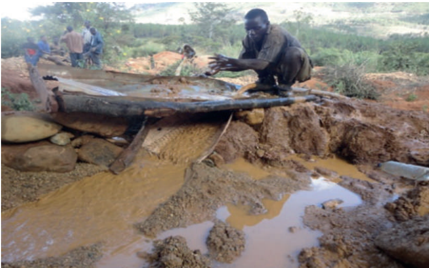
FIGURE 4 | HOME MADE SLUICES FOR GOLD RECOVERY IN MANICA, MOZAMBIQUE
