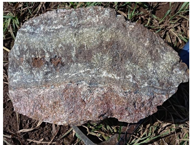
Monazite-rich vein and its brown altered exocontact in carbonatite, the top of the Kangankunde Hill.
