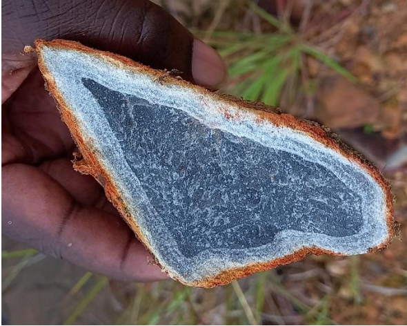
Massive phonolite fragment showing contrasting and zoned weathering crust. Liwonde, Nsanama road.
