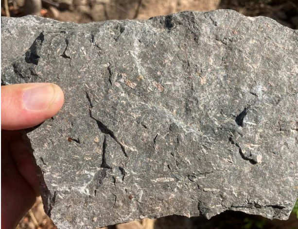
Fine-grained trachyte. Liwonde West area.
