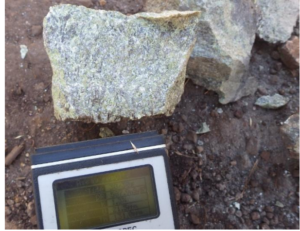
Figure 29: Gamma-ray spectrometry measurement in Kangankunde, showing slightly elevated signature of thorium and potassium.
