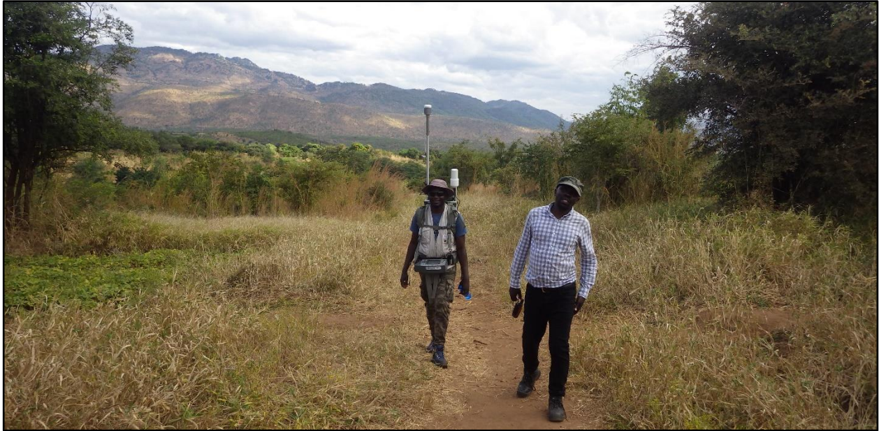
Figure 24: Data acquisition using G-859 Caesium magnetometer by Chrispin Ngwata, with Brave Manda using the GPS for navigation.
