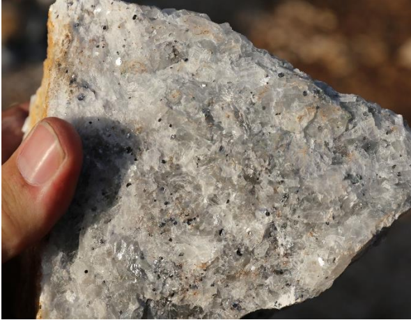
Coarse-grained graphite marble from the Zalco Quarry, Chiendausiku region.
