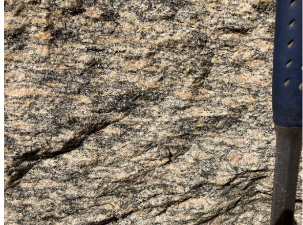
Augen orthogneiss, quarry WNW of Nsanama.
