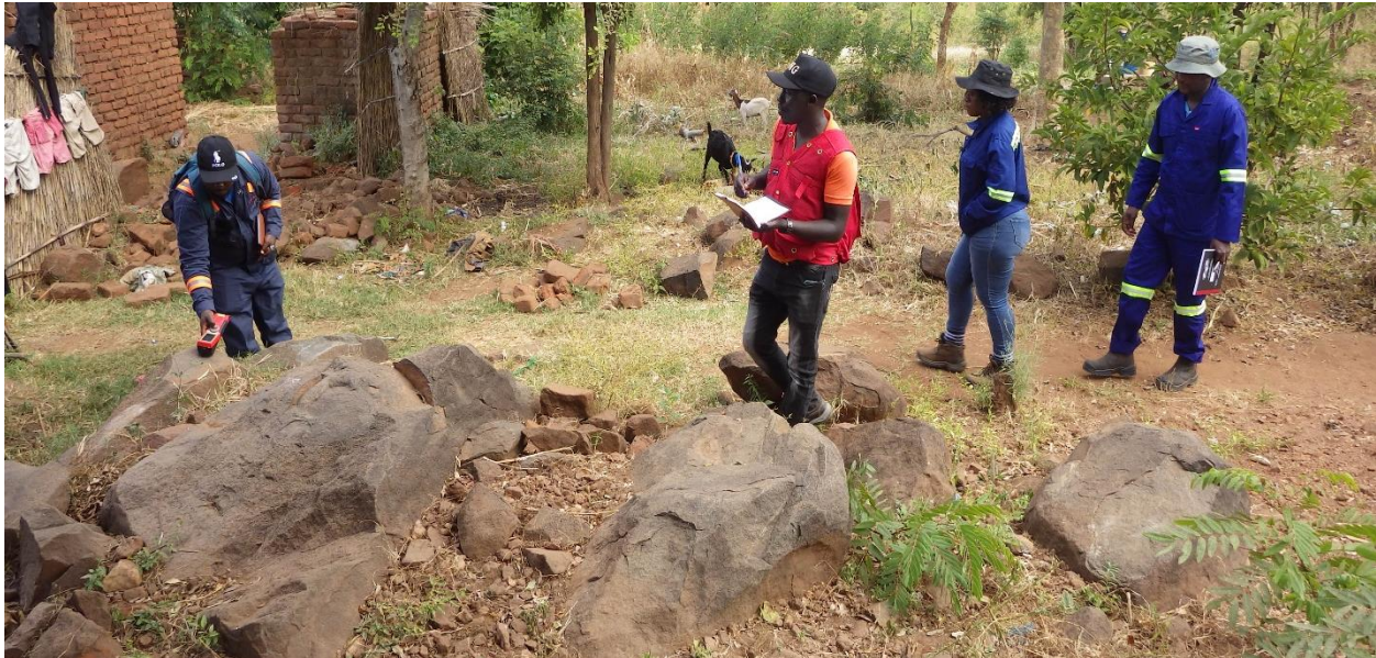
Figure 25: Some of the participants taking magnetic susceptibility measurements of the possibly Karoo dolerite dyke.
