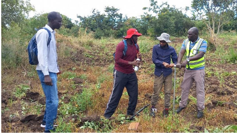
Figure 32: Soil sampling with the core soil bar for heavy soils, Liwonde-East.
