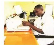
Polishing Machine for Polished Mount Preparation
