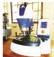
Polishing Machine for Polished Mount Preparation
