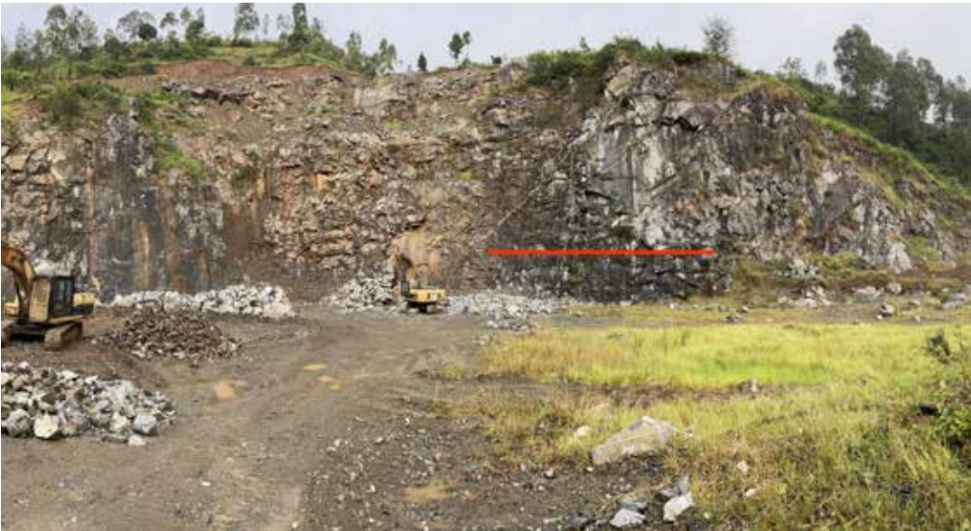
Figure 6 - Scanline in the rock slope outcropping in Gatumba Quarry
