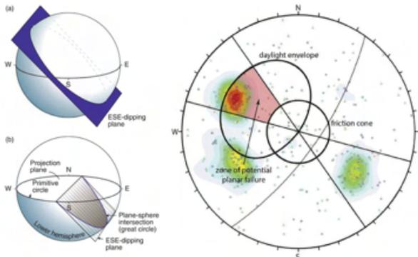
**Figure 21 - Stereographic projection and example of kinematic analysis**
