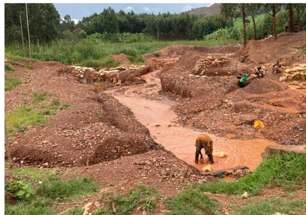
**Figure 34.** The ASM operation for alluvial tin placer beneath the Mwerasandu hill.
