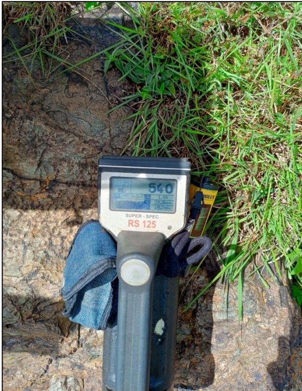
**Figure 18.** Gamma-ray spectrometry measurement in Assay mode
