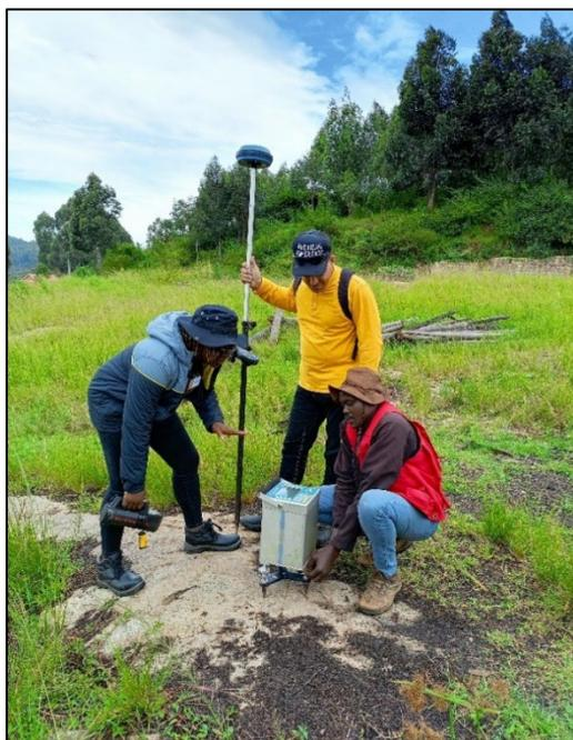
**Figure 16.** Levelling the gravimeter on its stand.
