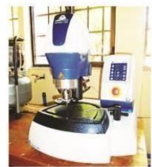
Polishing Machine for Polished Mount Preparation
