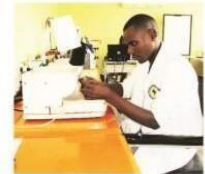
Polishing Machine for Polished Mount Preparation
